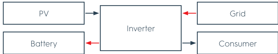
Figure 31 Solar energy not sufficient, additional energy for consumers from the grid
