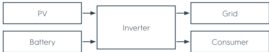
Figure 26 Battery charged, sufficient solar energy, surplus energy and energy from the battery into the grid
