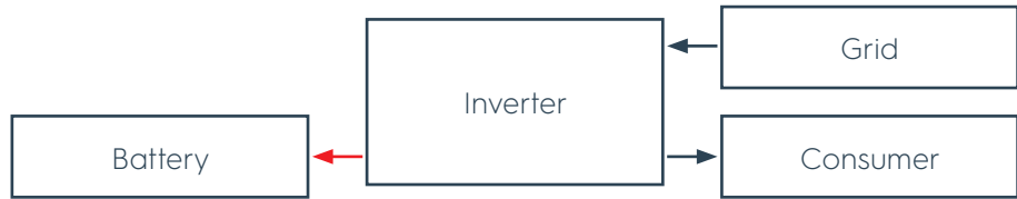
Figure 27 Energy for battery charging from the grid
