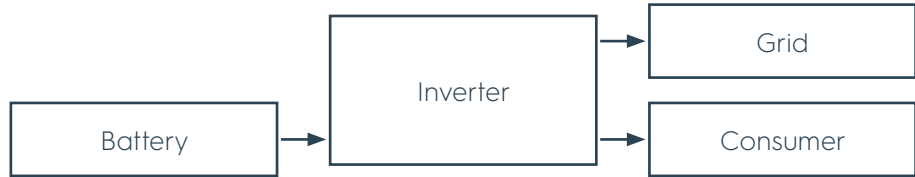
Figure 28 Energy from the battery sufficient, surplus energy into the grid
