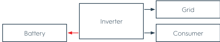
Figure 27 Energy for battery charging from the grid
