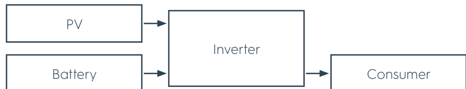
Figure 23 Solar energy not sufficient, additional energy from the battery
