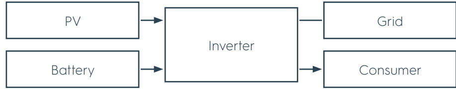
Figure 20 Solar energy not sufficient, additional energy from the battery
