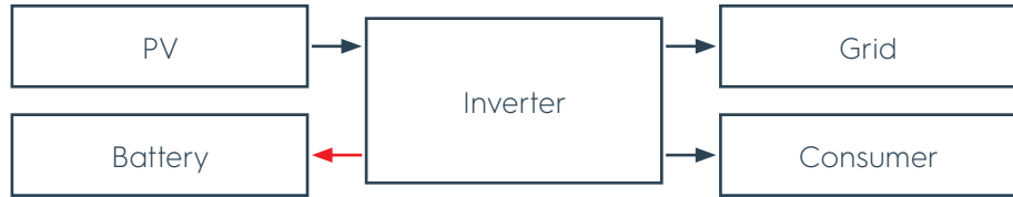
Figure 24 Sufficient solar energy, surplus energy for consumers and into the grid
