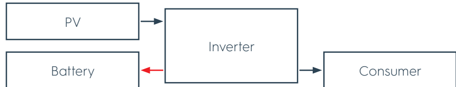
Figure 22 Sufficient solar energy, surplus energy for battery charging
