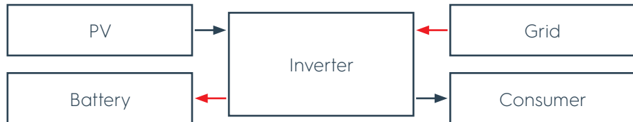
Figure 25 Solar energy not sufficient, additional energy for consumers from the grid
