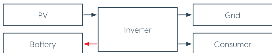
Figure 19 Sufficient solar energy, surplus energy for battery charging and into the grid
