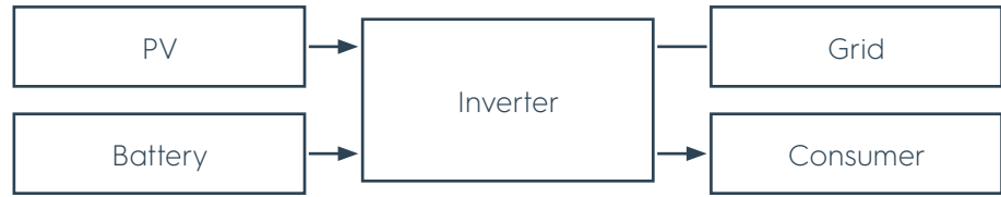
Figure 20 Solar energy not sufficient, additional energy from the battery
